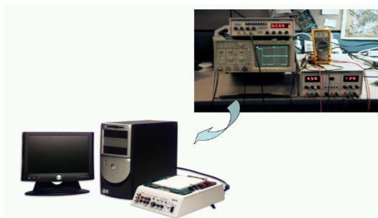
Figure 1: Appearance of a traditional measurement instrument and a virtual one.
